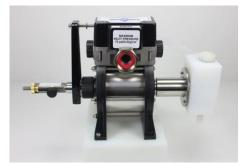
Model # MV6080-HDPE-TTE,DMAC Hydroblend Proportioner Max Ratio: 5.80% (8oz/gallon) Min Ratio: 0.60% Max Water Flow: 12 GPM @ 75 psi
