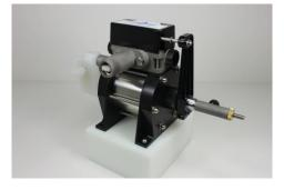
Please be aware that the above units are our Chlorine/Bleach specific proportioners. All units are configured with a SST Valve Block, Water Motor and Outlet Fitting. The chemical side of the pump is configured with an HDPE Pump Head, Viton seals, a chemically resistant Hastelloy Chemical Cylinder, and can be configured to mount on either a horizontal or a vertical surface.
