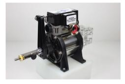
Please be aware that the above units are our Poultry specific proportioners. All units are configured with a SST Valve Block, Water Motor and Outlet Fitting. The chemical side of the pump is configured with an Acrylic Pump Head, Viton seals, and can be configured to mount on either a horizontal or a vertical surface.
