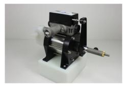
Please be aware that the above units are our PAA specific proportioners. All units are configured with a SST Valve Block, Water Motor and Outlet Fitting. The chemical side of the pump is configured with a Kynar Pump Head, PAA specific seals, hot water capable Delrin Machined Endplates (DMAC), and can be configured to mount on either a horizontal or a vertical surface.
