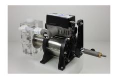
Please be aware that the above units are our 6000 Series (7 GPM) proportioners. All units are configured with a SST Valve Block, Water Motor and Outlet Fitting. The chemical side of the pump is configured with an Acrylic Pump Head, Viton seals, and can be configured to mount on either a horizontal or a vertical surface.
