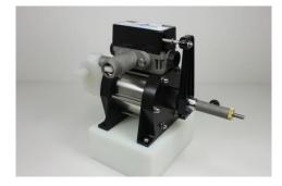
Model # 6020-HDPE-V,BLE Hydroblend Proportioner Max Ratio: 1.50% (2oz/gallon) Min Ratio: 0.15% Max Water Flow: 7 GPM @ 75 psi
