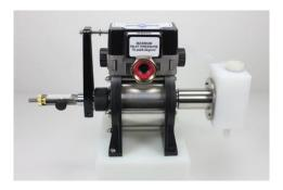
Please be aware that the above units are our Conveyor/Chain Lubricant specific proportioners. All units are configured with a SST Valve Block, Water Motor and Outlet Fitting. The chemical side of the pump is configured with a PVC Pump Head, Viton seals, and can be configured to mount on either a horizontal or a vertical surface.
