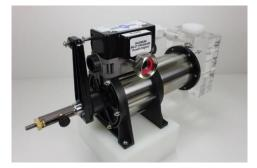
Please be aware that the above units are our 6000 Series (7 GPM) Silicone specific proportioners. All units are configured with a SST Valve Block, Water Motor and Outlet Fitting. The chemical side of the pump is configured with an Acrylic Pump Head, Viton seals, and can be configured to mount on either a horizontal or a vertical surface.
