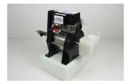
Please be aware that the above units are our High Dilution Cleaner specific proportioners. All units are configured with a SST Valve Block, Water Motor and Outlet Fitting. The chemical side of the pump is configured with a PVC Pump Head, EPDM seals, and can be configured to mount on either a horizontal or a vertical surface.
