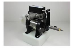
Please be aware that the above units are our 6000 Series (7 GPM) Chlorine specific proportioners. All units are configured with a SST Valve Block, Water Motor and Outlet Fitting. The chemical side of the pump is configured with an HDPE Pump Head, Viton seals, a Hastelloy Chemical Cylinder and can be configured to mount on either a horizontal or a vertical surface.
