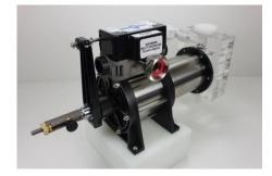
Please be aware that the above units are our 6000 Series (7 GPM) Emollient specific proportioners. All units are configured with a SST Valve Block, Water Motor and Outlet Fitting. The chemical side of the pump is configured with a PVC Pump Head, Viton seals, and can be configured to mount on either a horizontal or a vertical surface.
